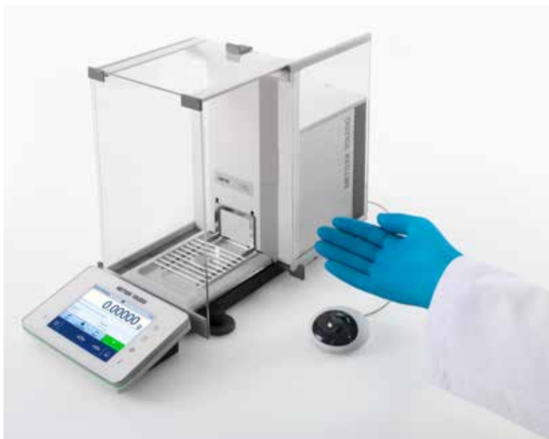
Figure 6: Operate the balance without touching it: Add an optical hand-sensor, configured to open the draft shield door, to tare or to print results simply with a wave of your hand.
