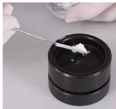
Figure 32. Filling the first portion of a solid sample
