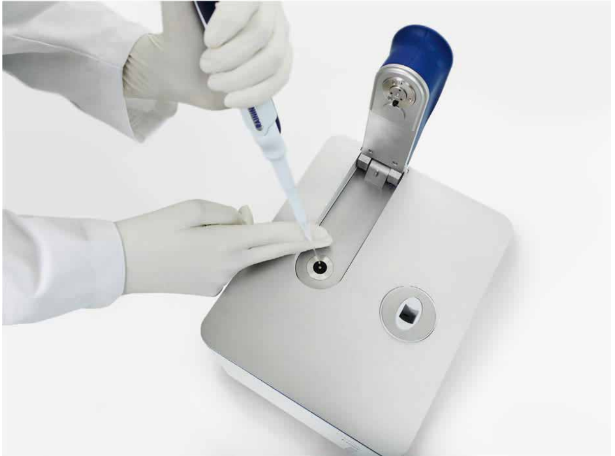
Figure 16. Sample is applied to the micro-volume platform with a micro-liter pipette
