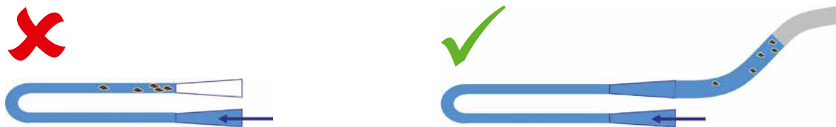
Figure 21. Filling of the density cell. Left: inappropriate. Right: good.
