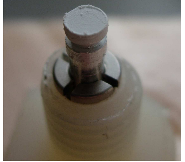
Figure 12: The third SEM target after the test, showing a thick coating of salt.
