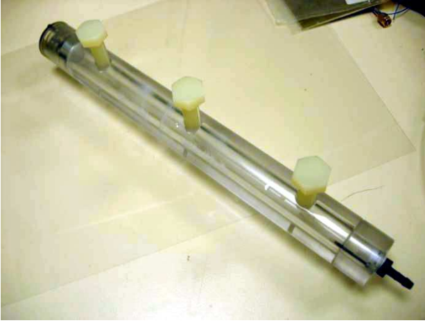
Figure 3: The electrostatic precipitator was machined from perspex, with a piston at the inlet to prevent contamination.
