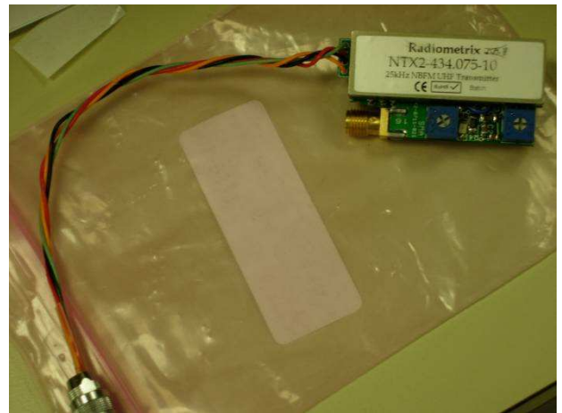
Figure 28: The assembled 434MHz radio datalink.
