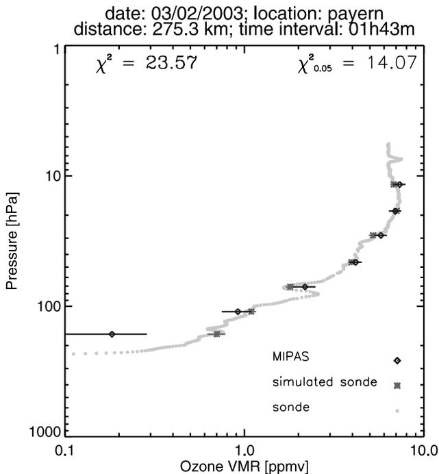
**Figure 4c.** Same as Figure 4a but with data acquired at Payerne on 3 February 2003 at 275.3 km distance and 1 hour 43 min time interval. Value of  $\chi^2$  with respect to the 5% threshold  $\chi_{0.05}^2$  for 7 degrees of freedom shows that MIPAS retrievals in the comparison are not validated.
