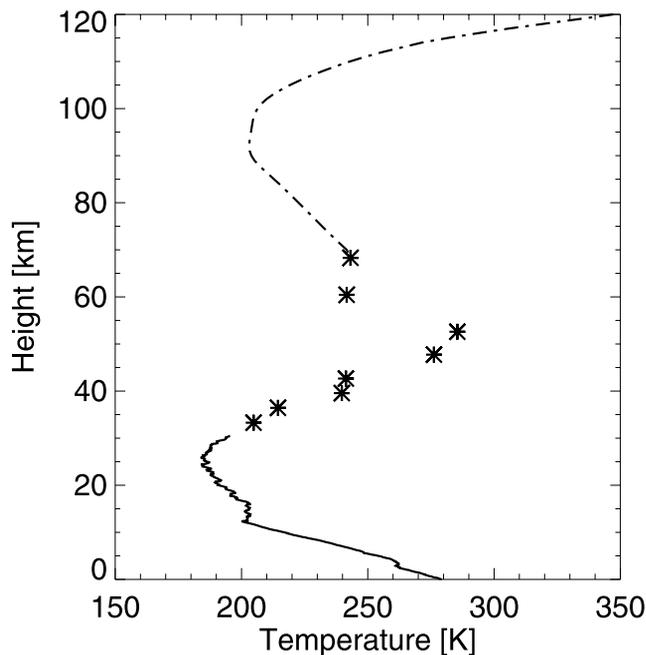
**Figure 2.** Temperature profile from 0 to 120 km as measured by a radiosonde in Ny-Ålesund on 7 December 2002 1200:51 UTC (solid line) and by MIPAS on 7 December 2002 1012:58 UTC from a distance of 234 km (asterisks). Temperature information in the upper part of the atmosphere (dash-dotted line) is taken from a climatology of the Arctic region in January, which was smoothly joined to the MIPAS retrieval (see text).
