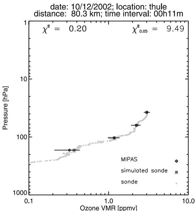
**Figure 4a.** Comparison between MIPAS ozone retrievals (open diamonds) and MIPAS ozone simulated retrievals (asterisks) using sonde ozone profiles (dots). Data were acquired at Thule on 10 December 2003 at 80.3 km distance and 0 hours 11 min time interval. Value of  $\chi^2$  with respect to the 5% threshold  $\chi_{0.05}^2$  for 4 degrees of freedom shows that MIPAS retrievals in comparison are validated.
