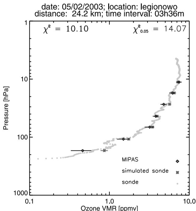
**Figure 4b.** Same as Figure 4a but with data acquired at Legionowo on 5 February 2003 at 24.2 km distance and 3 hours 36 min time interval. Value of  $\chi^2$  with respect to the 5% threshold  $\chi_{0.05}^2$  for 7 degrees of freedom shows that MIPAS retrievals in the comparison are validated.
