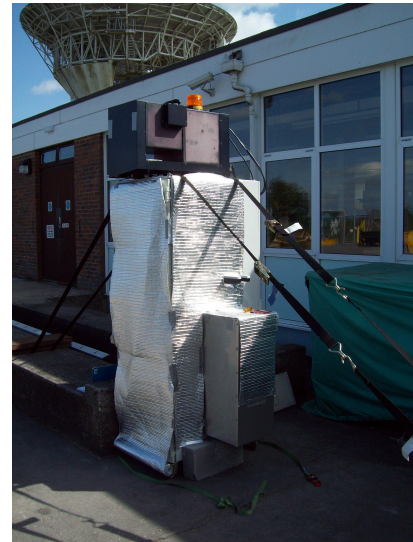
Figure 1. RACHEL deployed at the Chilbolton Observatory in southern England. Reflective insulation has been applied to the surfaces exposed to direct sunlight to improve temperature stability.
