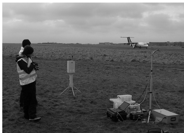
Figure 6. FAAM aircraft taxiing to takeoff at Cranfield, 17/2/09. The inputs to the Grimm samplers are on the stand to the right of the photograph. The Lidar is 375 m to the right of the frame; it was aligned on the Osiris, which is the instrument standing in the center of the photograph.
