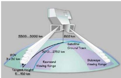
In normal operation MIPAS views rearward along the orbit track giving pole-to-pole coverage and approximately 14 orbits per day. It scans in elevation to acquire a set of limb emission spectra from tangent altitudes from approximately 70km (mesosphere) down to 6km (troposphere) every few hundred km along the orbit track.
