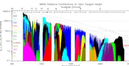
Above is a simulated MIPAS spectrum for a tangent height of 12km showing the spectral features associated with the atmosphere's main infrared emitting species in the 5 MIPAS bands. It is not essential to use a spectrally resolving instrument to retrieve most of these species, although doing so does improve accuracy.
