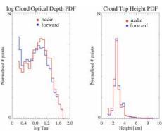
Using the forward-view radiances results in a greater proportion of optically thin cloud being detected. Similarly, a slightly greater proportion of high cloud is detected when the forward view radiances are used. Incorporating the forward view radiances into the retrieval scheme may improve the retrieval of Cirrus cloud. Further work is required to correctly collocate the properties derived using the different radiance measurements.
