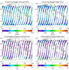
The maps above show the retrieved cloud top height and cloud optical depth for the 1<sup>st</sup> October 2000, as retrieved by ATSR-GRAPE using the forward-view and nadir-view radiances respectively. The results are gridded at 1° x 1° resolution. The results of using the different viewing geometries are compared in the histograms below.
