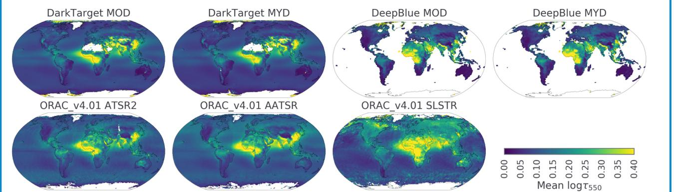
Figure 3 (above): All-time averages of log AOT at 550 nm for the ORAC, Dark Target and Deep Blue algorithms with various sensors. Though work remains to reduce noise in the ORAC SLSTR aerosol product, especially near the poles, it exhibits a number of useful properties: lower AOT over remote ocean which is more consistent with the MODIS products, reduced sensitivity to mountains, and higher AOT over the Arabian peninsula.
