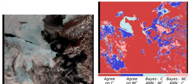
Figure 2: Comparing the new neural net cloud mask to a Bayesian classification (right), over a complicated scene (shown in false-colour below left) shows the new mask is better at identifying bright surfaces as not cloud (NC), though more work is needed.
