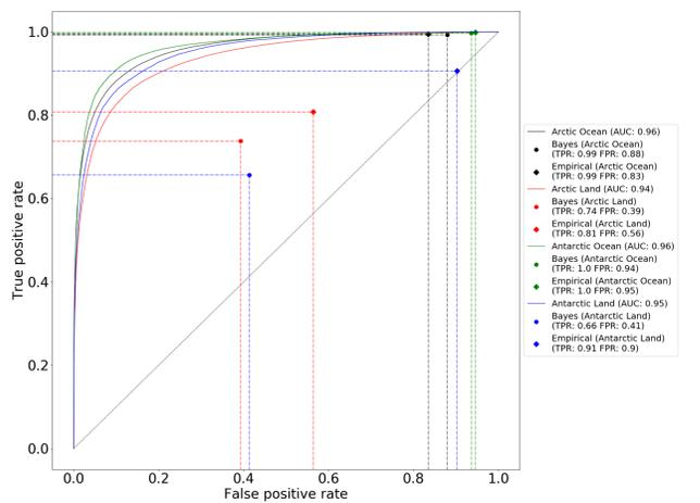
Figure 1: A cloud masking neural network can be tuned to balance the true and false positive rates (lines), achieving better performance than our existing methods (dots) in a variety of environments (colours).
