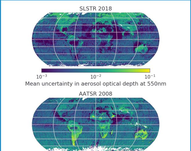
Figure 6: The mean uncertainty in aerosol optical depth from SLSTR during 2018 (top) and AATSR during 2008 (bottom). Uncertainties over the Southern Hemisphere land have decreased while those over Northern Hemisphere land have increased because of the switch from a forward to a reverse view between instruments changing the scattering angle observed.
