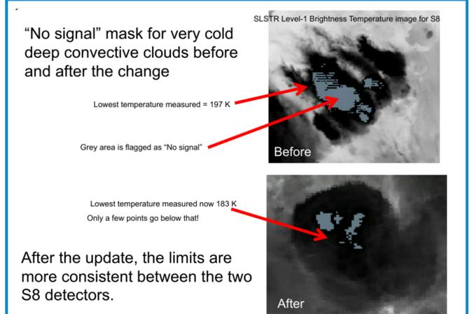
Figure 7: Working with the SLSTR calibration team, the dynamic range of the thermal channels was adjusted to resolve the cold tops of deep convective clouds on both Sentinel-3 A and B.
