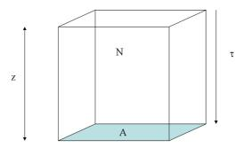
area is A. If  $\rho$  is the density of the aerosol and Z is the height of this volume then the total mass of aerosol, M, in the box is given by
