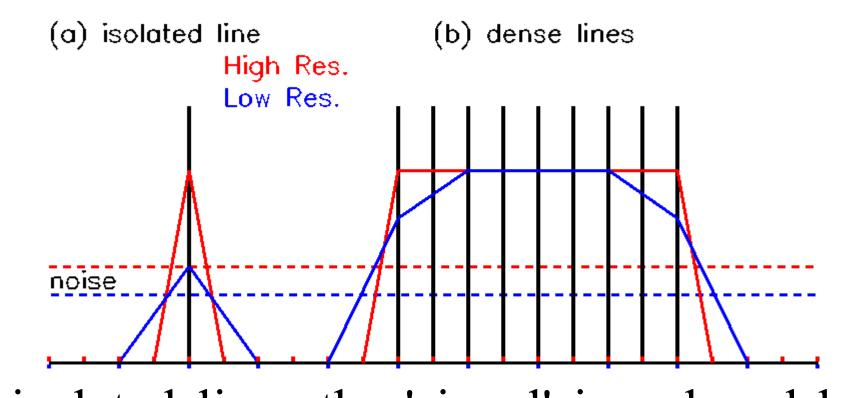
For isolated lines the 'signal' is reduced by a factor R while for dense features it remains constant.
