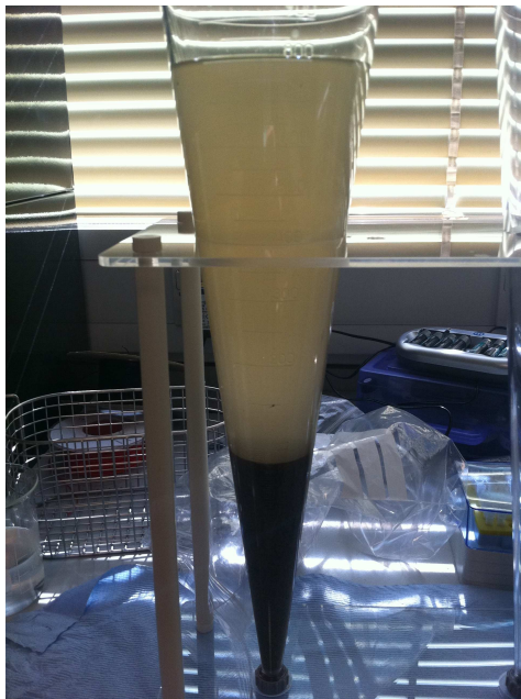
Figure 4.12: Imhoff cone containing the commercial sand in distilled water after 24 hours of settling. It can be seen that a considerable mass of coarse material has accumulated at the bottom, leaving the finer material still in suspension.
