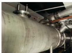
Long path-length absorption cell for broadband quantitative measurements from 32 m to over 1 km optical path
