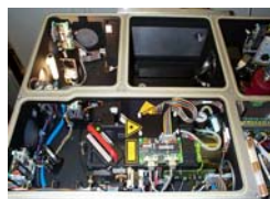
The Bruker IFS 66v/S FTS for measurements requiring moderate spectral resolution
