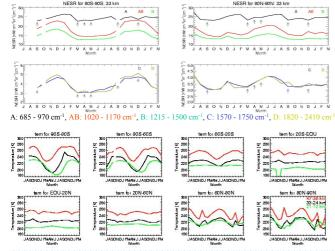
The NESR varies with time, steadily rising between decontamination events (shown by arrows in top panels). The effect of this ice decontamination is a reduction of the gain increase and of the noise level. This time dependence contribution to the predicted random error also depends on the atmospheric temperature, which controls the total radiance received.
