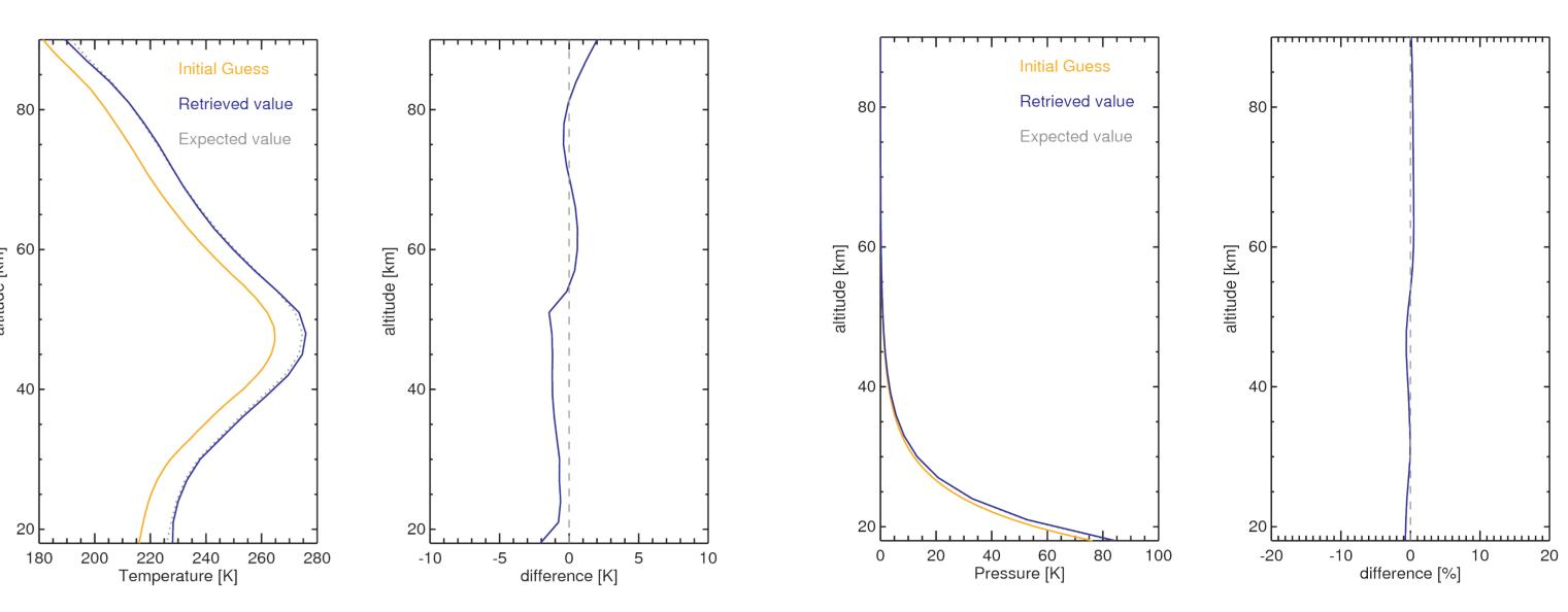
The simulations presented in the previous sections suggest that it should be feasible to retrieve pressure and temperature linearly assuming that the expected value is not too far from the linearization point (the initial guess). When dealing with real measurements the altitudes derived from the on board pointing knowledge will provide an additional piece of information to constrain the temperature and pressure retrieval via the hydrostatic equation, therefore improving these retrievals.
