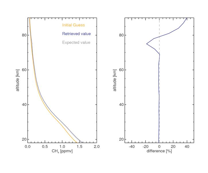
These results suggest that at least the retrievals of gas concentration can be done linearly in a single iteration without running the forward model during the inversion scheme. However, before retrieving any gas concentration it is necessary to know the atmospheric temperature and pressure.
