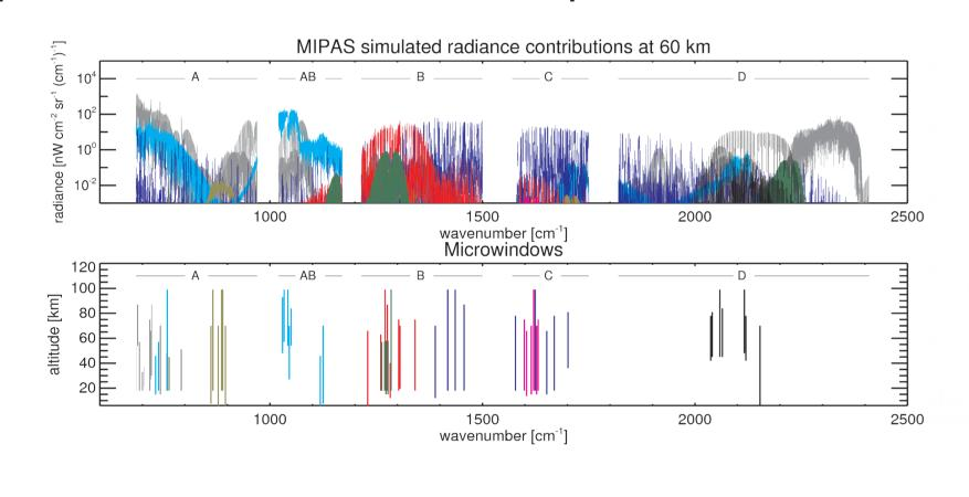
These Microwindows are currently the MIPAS Orbital Retrieval Sequential using Estimation (MORSE) developed in Oxford University for the MA observations.
