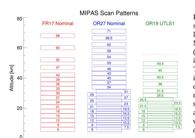
Projection of various MIPAS scan patterns onto the atmospheric limb. Rectangles represent the MIPAS effective field-of-view (30x10km), shown to scale. Numbers indicate the nominal tangent heights. The OR27 and OR19 scan patterns included a latitude-dependent altitude offset (dotted lines showing max/min range) following the tropopause shape. Although the limb is sampled at 1.5km spacing, the achievable vertical resolution in the L2 data is approx 2km at best.
