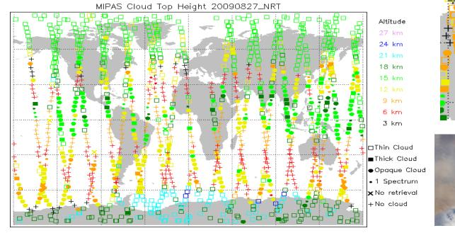
The main plot above shows the cloud retrieval results for 27 Aug 2009. Apart from the expected Polar Stratospheric Clouds at high altitude in the Antarctic, this also shows a uniform 'thin cloud' coverage at around 15km altitude throughout the Arctic. Working
