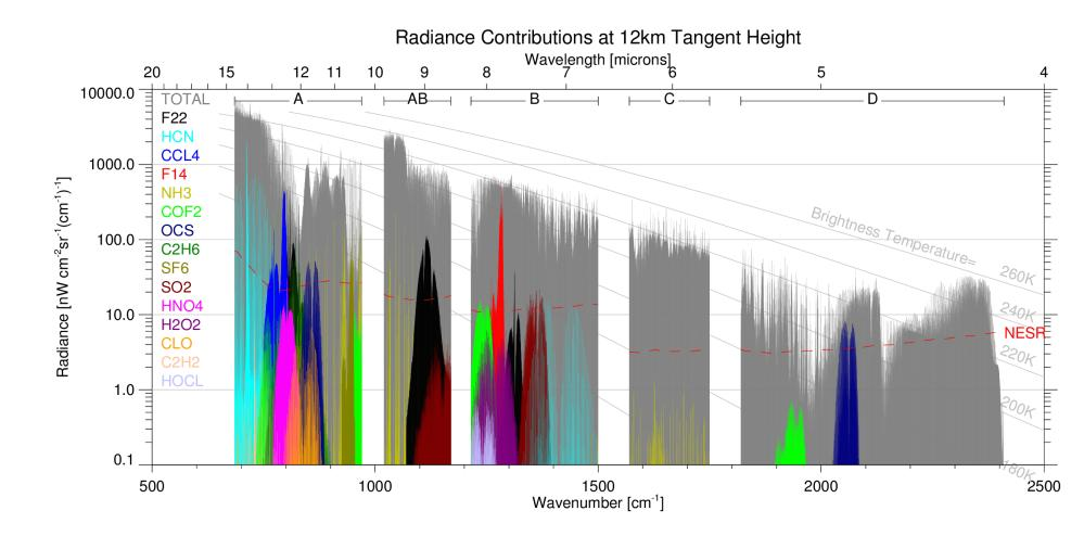
Above is a plot showing spectral signatures of minor species. High spectral resolution *is* essential in order to discriminate emission features of these molecules from the stronger emitters (shown in gray)
