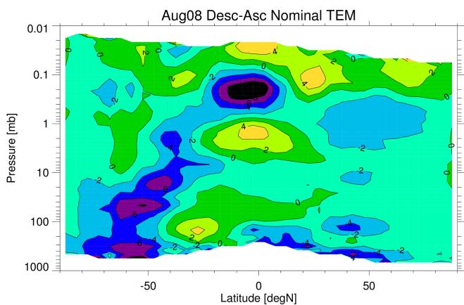
The plot above shows the difference in zonal mean temperature for August 2008 between the descending (day-time) and ascending (night-time) orbits. The oscillating structure over the equator is the (real) diurnal tide. However the differences at mid-latitudes are thought to arise from neglecting horizontal temperature gradients in the retrieval forward model. Similar artefacts can be seen in the day-night differences of most species in the Oxford (and ESA) data.
