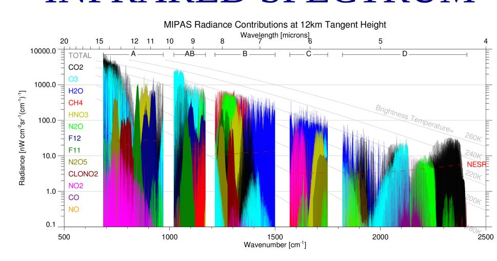
Above is a simulated MIPAS spectrum for a tangent height of 12km showing the spectral features associated with the atmosphere's main infrared emitting species in the 5 MIPAS bands. It is not essential to use a spectrally resolving instrument to retrieve most of these species, although doing so does improve accuracy. Below is a plot showing the spectral features of minor species examined here. High spectral resolution *is* essential to separate these from the major absorbers.
