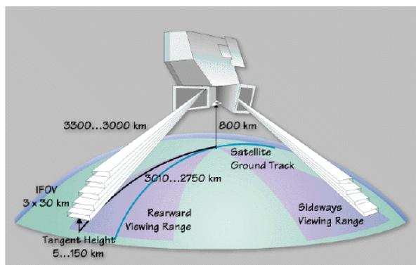
In normal operation MIPAS viewed rearward along the orbit track giving pole-to-pole coverage and approximately 14 orbits per day. It scanned in elevation to acquire a set of limb emission spectra from tangent altitudes from approximately 70km (mesosphere) down to 6km (troposphere) every few hundred km along the orbit track.
