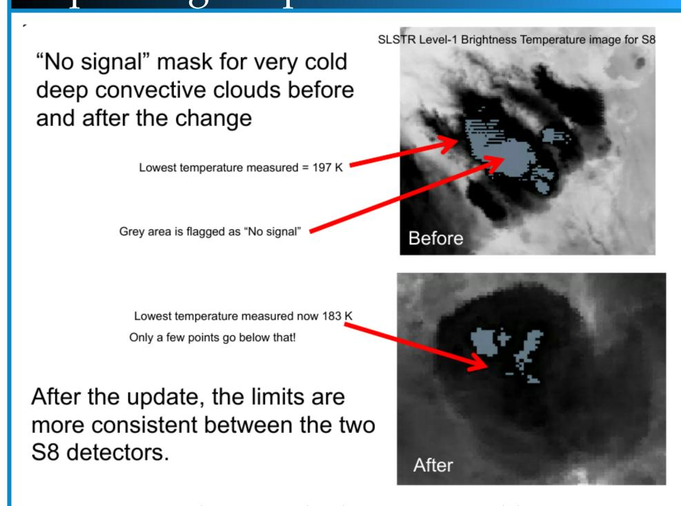
Figure 7: Working with the SLSTR calibration team, the dynamic range of the thermal channels was adjusted to resolve the cold tops of deep convective clouds on both Sentinel-3 A and B.
