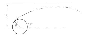
3. Two masses m and  $\delta m$  ( $\delta m \ll m$ ) are joined together, and moving with velocity v in some inertial frame. At some instant the mass  $\delta m$  flies apart from m (e.g. because of the release of a spring) along the direction of motion with a relative velocity w with respect to the mass m, such that the velocity of m becomes  $v + \delta v$ . Show that, if the small mass is projected in the backwards direction,
