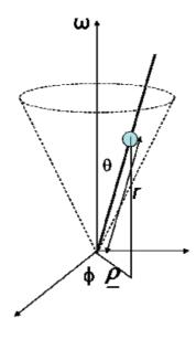
A bead of mass m is constrained to slide on a frictionless wire which is made to rotate about a vertical axis at an angular velocity  $\omega$ . The wire is tilted away from the vertical by a fixed angle  $\theta$  and the location of the bead is measured by the coordinate r.
