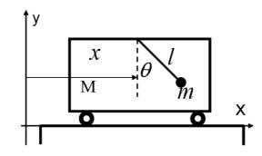
A box of mass M can slide horizontally on a frictionless surface. A simple pendulum of string length l and mass m, is suspended inside the block. Denote the coordinate of the centre of mass of the box by x and the angle that the pendulum makes with the vertical by  $\theta$ . At t = 0the pendulum displacement is  $\theta = \theta_0 \neq 0$
