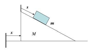
A block of mass m slides on a frictionless inclined plane of mass M, which itself rests on a horizontal frictionless surface.
